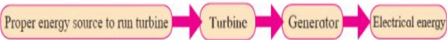
5.4 Flow chart showing generation of electrical energy
